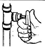
2 Turn "OFF" the water to the water heater. Some installations require that the water be turned off to the entire house.
